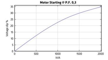
Peak motor starting (kVA) based on x% voltage dip power factor at 0.3
