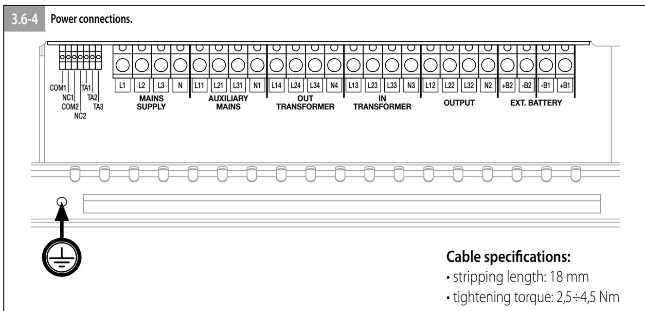
**3/3 MAINS AND AUXILIARY MAINS ARE CONNECTED SEPARATELY. Output transformer (standard configuration)**
