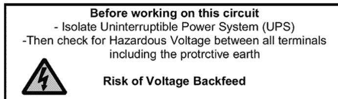
To install the external back-feed protection it is necessary to connect an external electromechanical switch. For further information on the connection and the type of remote switch, please read paragraph 11.6 of this manual.
