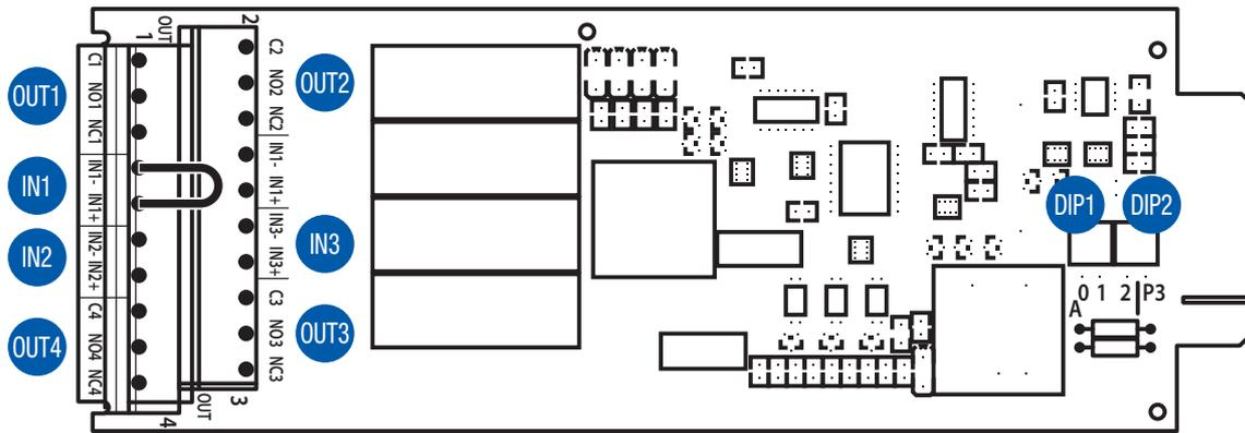
The filter level indicates the activation delay: **1** immediate activation (1 seconds minimum communication time), **2** 10 s delay, **3** 30 s delay.
