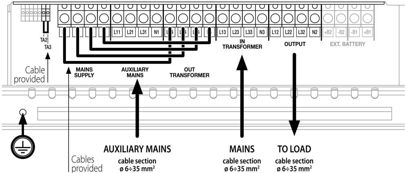
3/3 MAINS AND AUXILIARY MAINS ARE CONNECTED SEPARATELY. Transformer on the bypass power supply input
