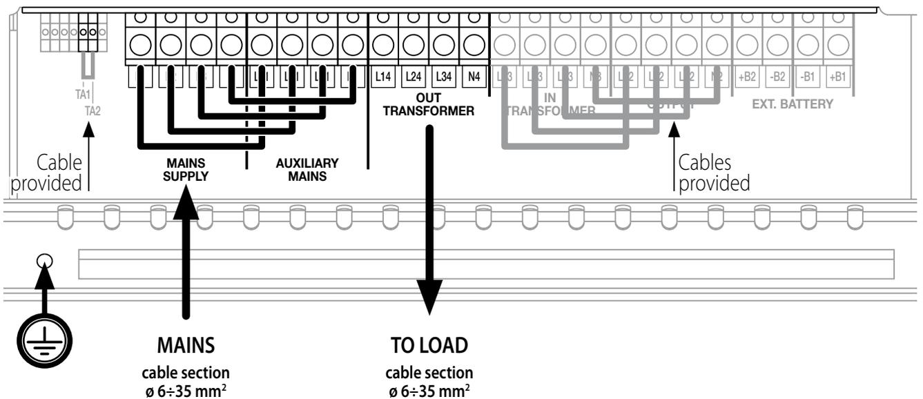
3/3 MAINS AND AUXILIARY MAINS ARE CONNECTED SEPARATELY. Transformer on the rectifier power supply input
