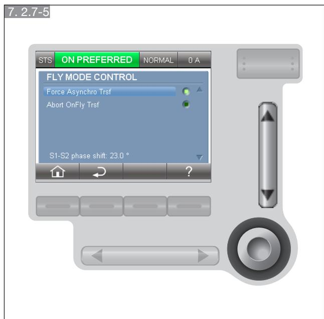
If sources are asynchronous, you can force the transfer or waiting for the transfer to occur automatically once the 2 sources become synchronous.
