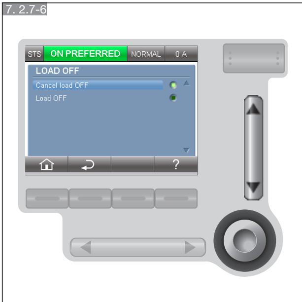
To switch off the load, press on the DOWN button, ENTER button and validate your choice .
