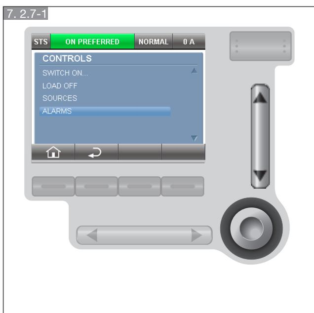
Press on the ENTER button to go on the “SWITCH ON...” menu.
